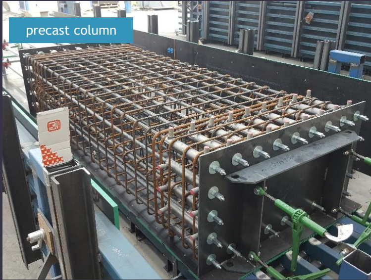
rebar cage with grout splices
