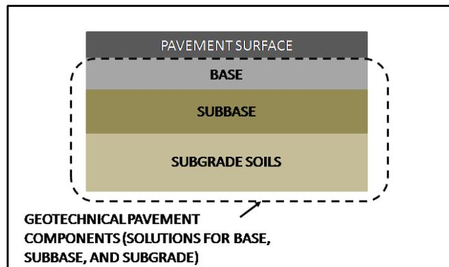
Geotechnical pavement components
