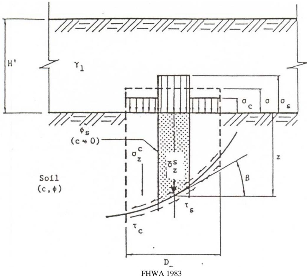
**Figure 5-22. Notation used in average stress method stability analysis.**
