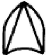
**EXCLUSIVE OR** – Output fault occurs if exactly one of the input faults occurs
