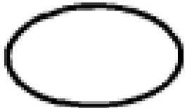
**CONDITIONING EVENT** – Specific conditions or restrictions that apply to any logic gate (used primarily with **PRIORITY AND** and **INHIBIT** gates)
