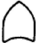
**OR** – Output fault occurs if at least one of the input faults occurs
