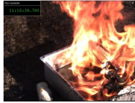
Cell immersed in synthetic ester: (a) before venting, (b) intensive venting, (c) fire generation during the explosion, (d) flames after in-tense venting.
