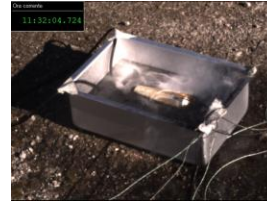
Cell immersed in Galden HT170 sequence a) before venting b) loss of bottom due to venting c) intensive venting d) after intense venting.
