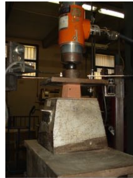
Fig. 12. Setup for the uniaxial compression test.
