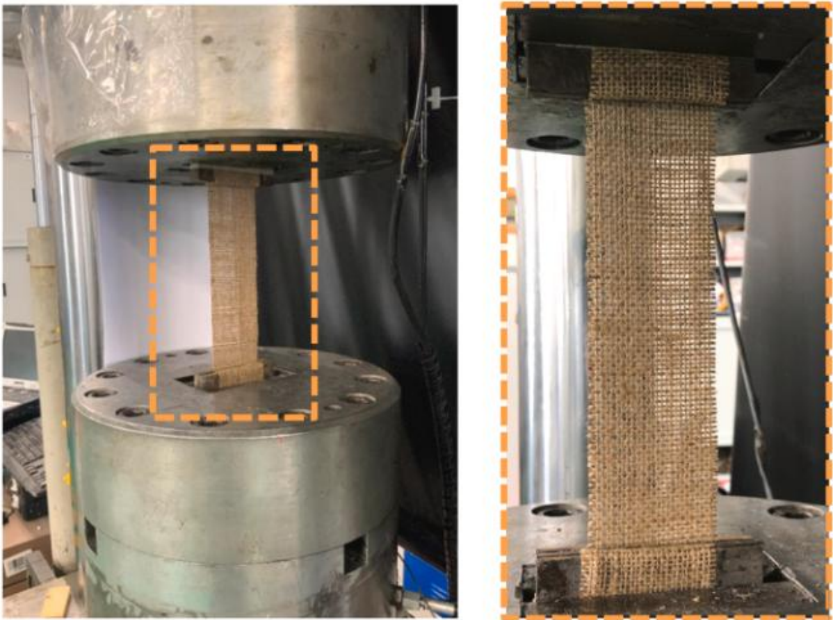
Fig. 3. Representative tensile test on natural textile: Jute.
