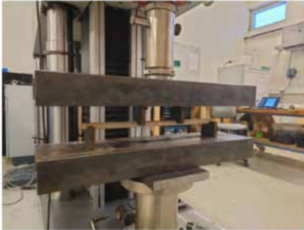
(b) Bending setup
