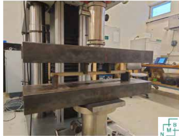
(b) Bending setup
