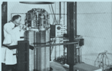
Geel, 1969 – The accelerator was an essential piece of equipment used in the study of neutron data, knowledge of which was fundamental especially to develop fast reactors.
